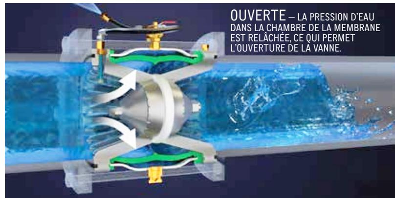
**OUVERTE** – LA PRESSIION D'EAU DANS LA CHAMBRE DE LA MEMBRANE EST RELÂCHÉE, CE QUI PERMET L'OUVERTURE DE LA VANNE.
